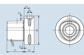
Widespread at multitask (mill-turn centers) machines. Torque transmission and centering due to polygon taper. Exact positioning by face contact. Very high static stiffness.
